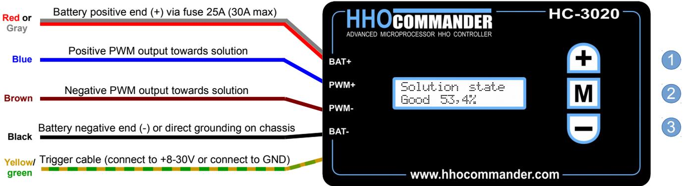
\*The fuse must be located in a easily accessible location near the battery's positive end for immediate removal
